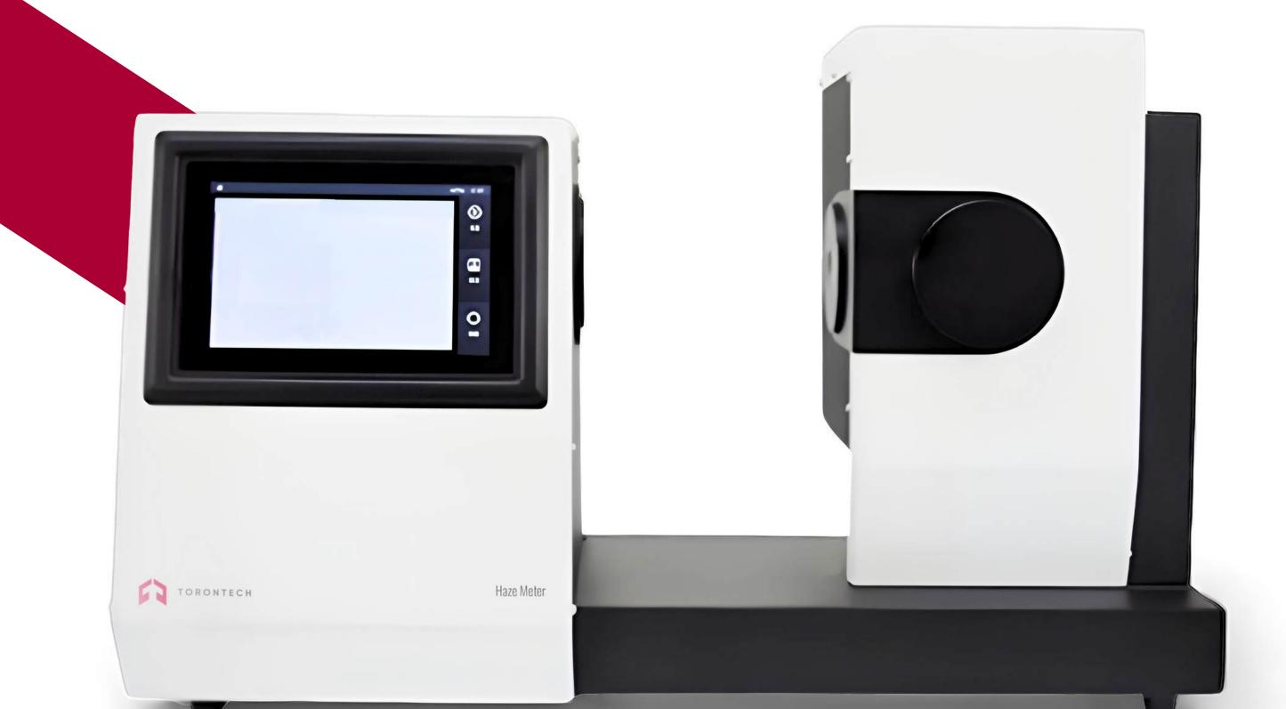
The Haze Meters are designed for accurate color, haze, and transmittance measurements, ideal for plastics, films, glass, LCD panels, touch screens, and other transparent or semi-transparent materials.
