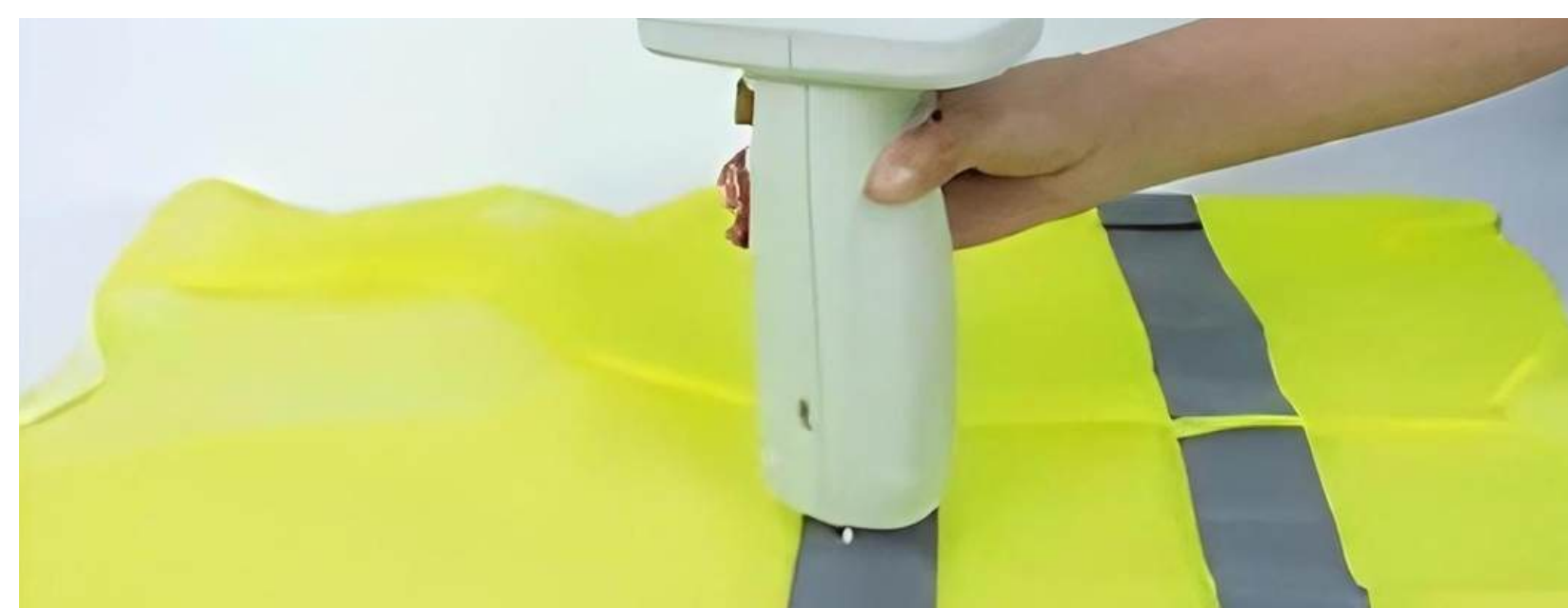
Measuring fluorescence color
