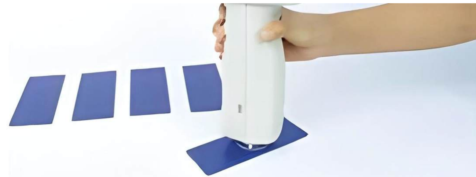
Measuring color difference of plastic sheets
