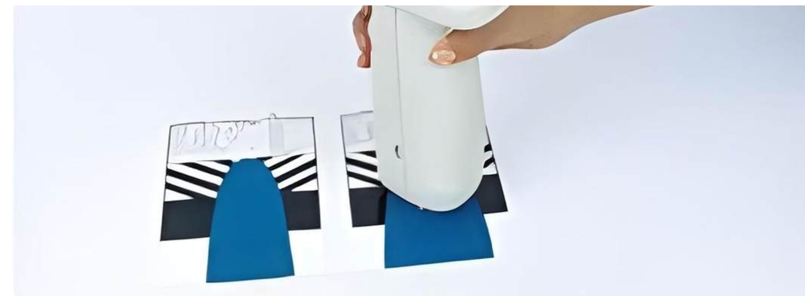
Measuring Coating Coverage
