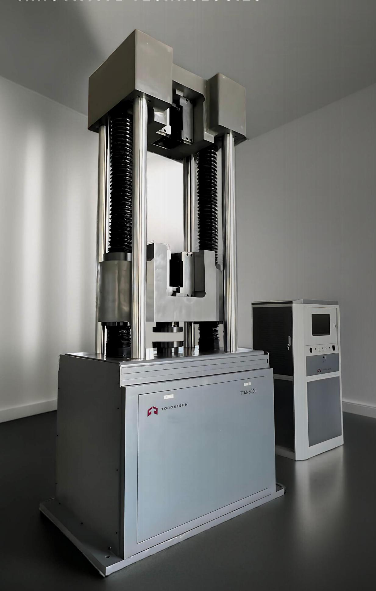
3000kN Hydraulic Universal Testing Machine TTM-3000
